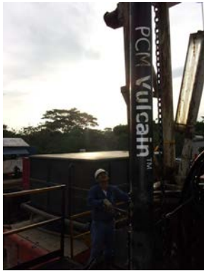
Figure 11: Running of PCM Vulcain™ Stator at well A
