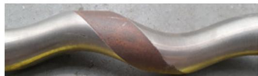
*Note: difference between abrasion and metal/metal wear: abrasion wear is round on sealing line while metal/metal wear generate a flat surface on sealing line.*
